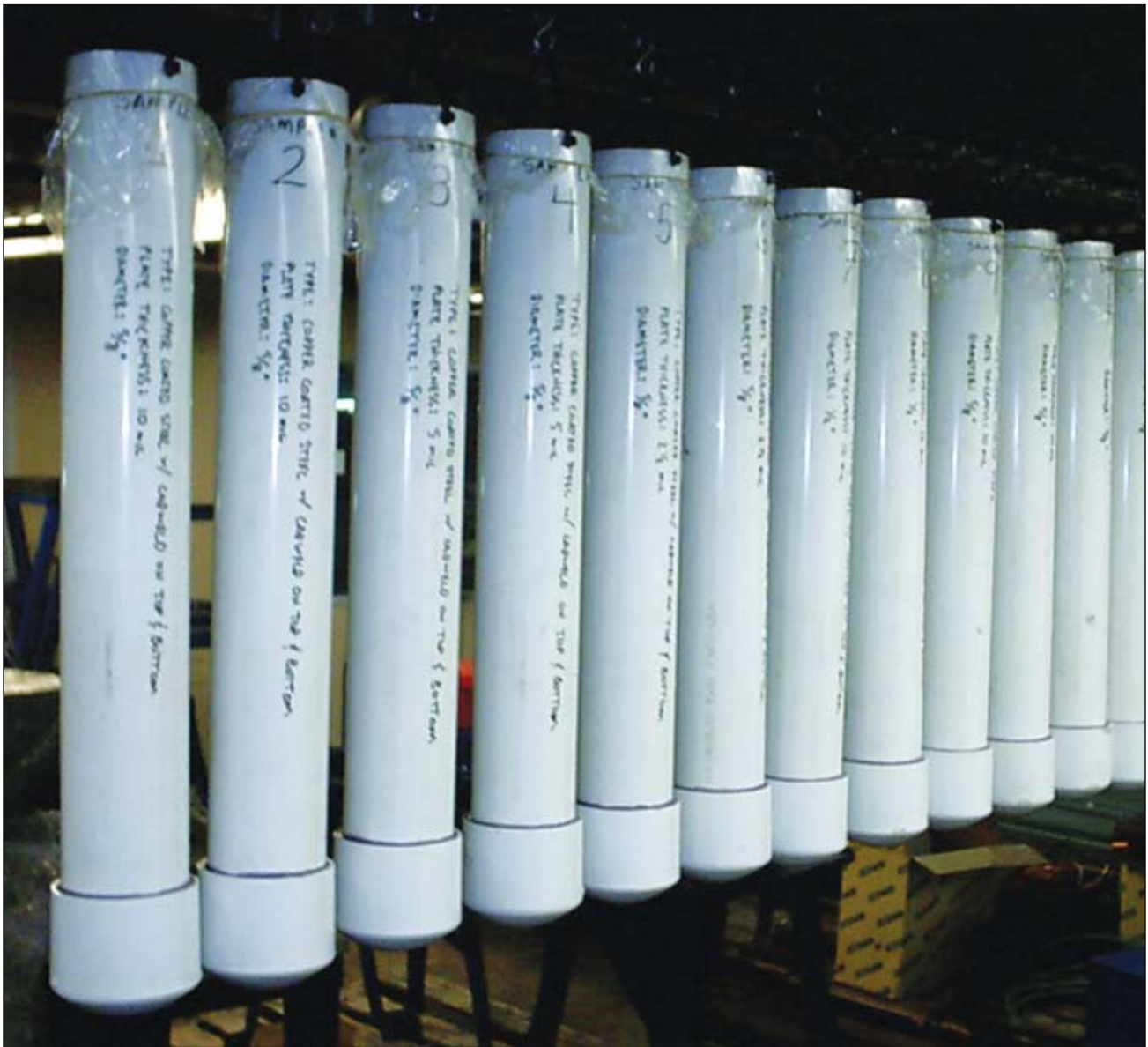
Photo 3. Line-up of ground rod samples in labelled PVC tubes
