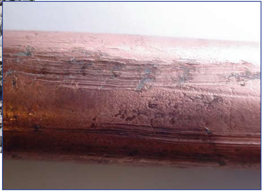
Photo 1(b). Typical “installation damage” to the ground rod coating
